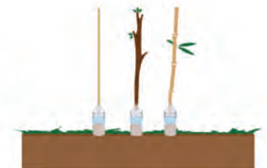
Wooden sticks held up by bottles filled with sand and/or water
